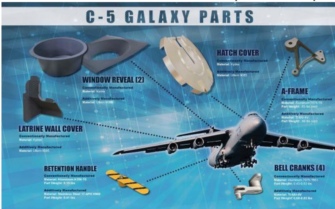
Figure 4: Expansion of the use of AM within the C-5 Galaxy Program. PA Case No. 78ABW-2020-0016(20-02391) Distribution A. Approved for public release.
