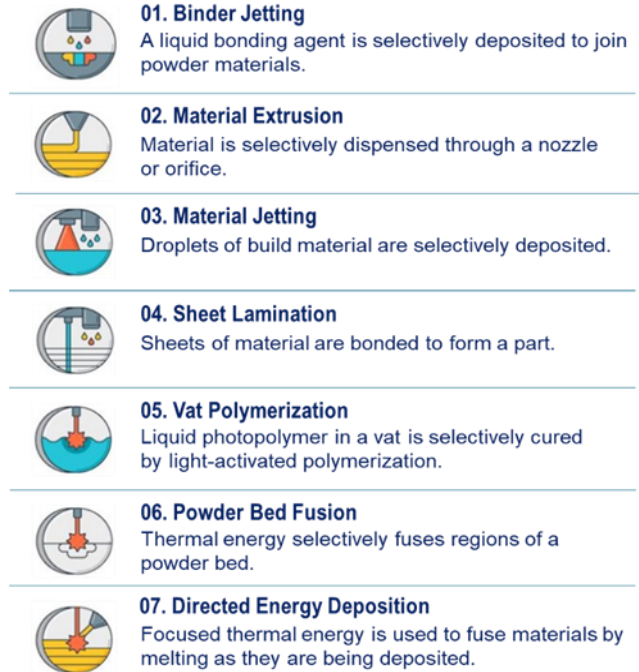
Figure 1: Seven industry recognized types of additive manufacturing processes (image courtesy of ASTM International).
