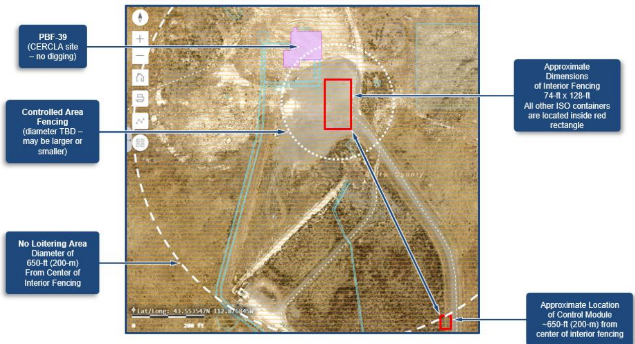
Figure 2. Conceptual Layout of the Mobile Microreactor at CITRC Pad A (from Nelson, 2023a)
