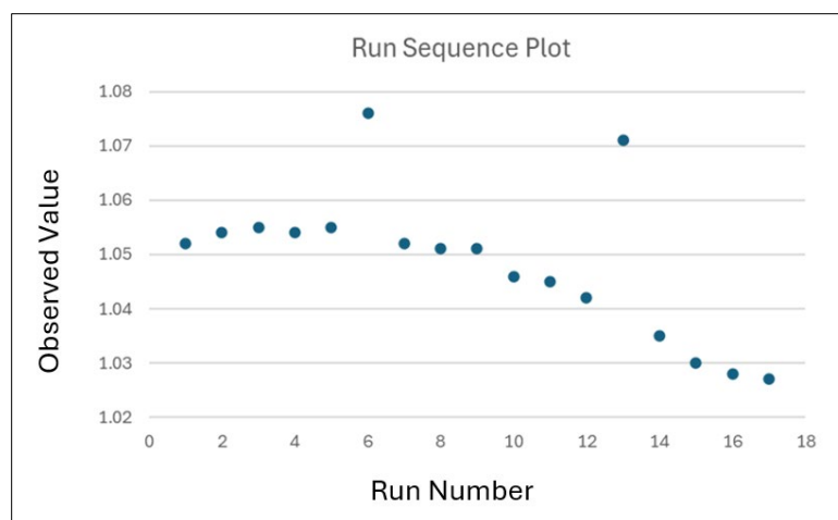
Figure 4-2. Run-Sequence Plot Showing an Overall Trend in Observations Along With Two Outliers
